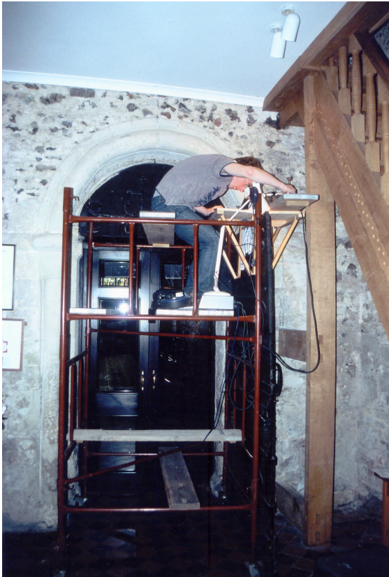
Fig 18 Great Door at St Peter's church, Old Woking. Andy Moir measuring the tree rings, having sanded down the top edge to expose them.
